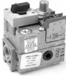
Used on gas fired standing pilot appliances with 30 mV thermocouple. These gas controls include a manual gas valve, safety shutoff, single millivoltage automatic operator, pressure regulator, pilot gas filter and flow adjustment, pressure tapping, and thermocouple connector.
